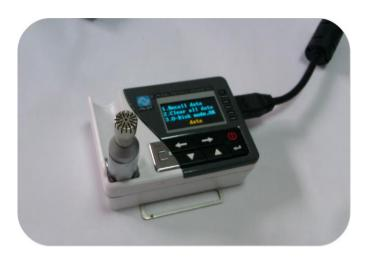
∞ The ASV 5910-1 model features ---dual dosimeters, datalogging/time history and 2GB storage.
